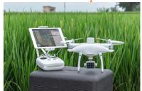
It is a high-precision integrated unit; Its time and space synchronization system, Centimeter-level positioning system and Integrated Spectral Sunlight Sensor ensure the accuracy of the data in the scanning area, which is a feature that ordinary multispectral cameras do not have.
